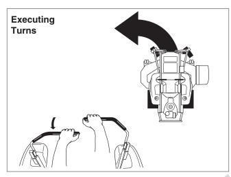
Figure 6. Turning Around a Corner
